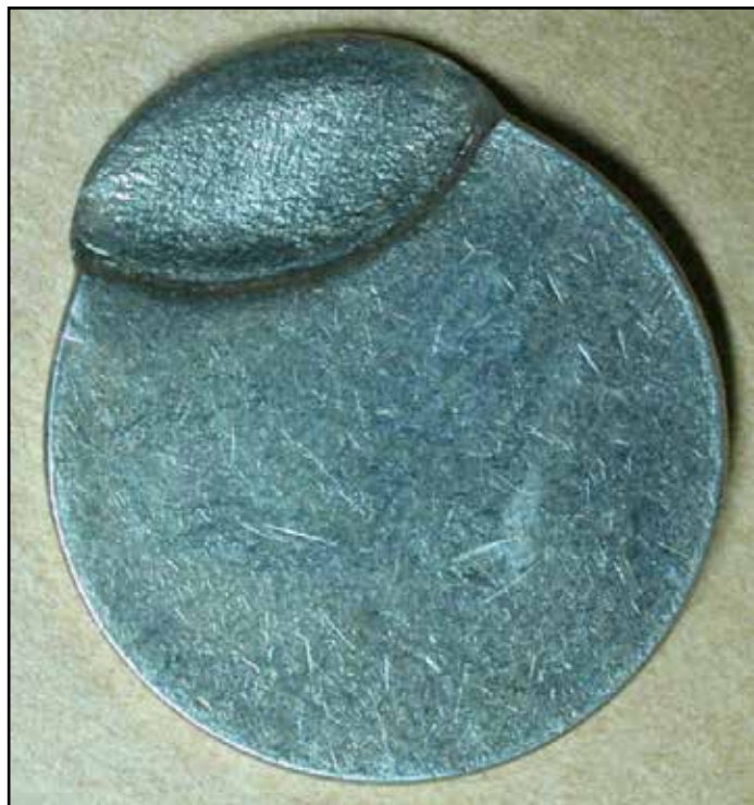
The obverse shows an indent from an unstruck planchet.
