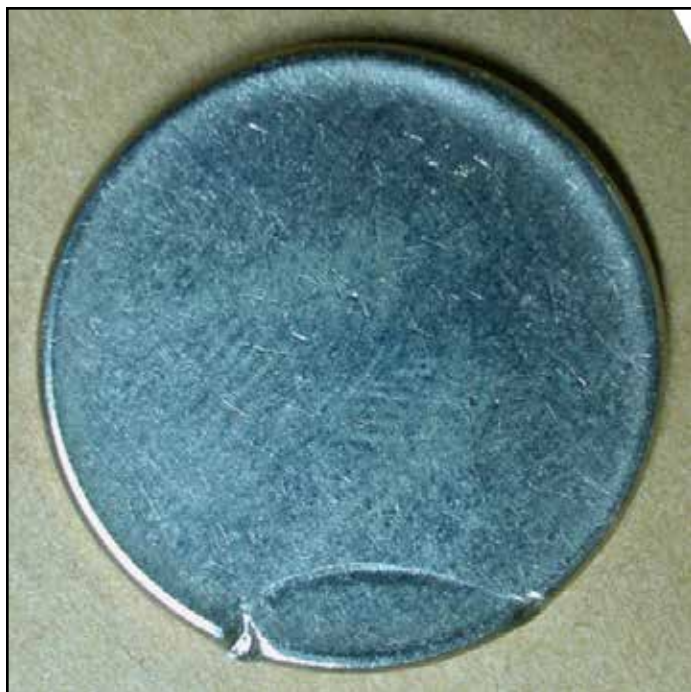
Shallow groove on the obverse of a 2005 West Virginia quarter with an “invisible strike”. This strike-through error is probably from a machine part or piece of hardware. Coin discovered by Gregory Capps.
