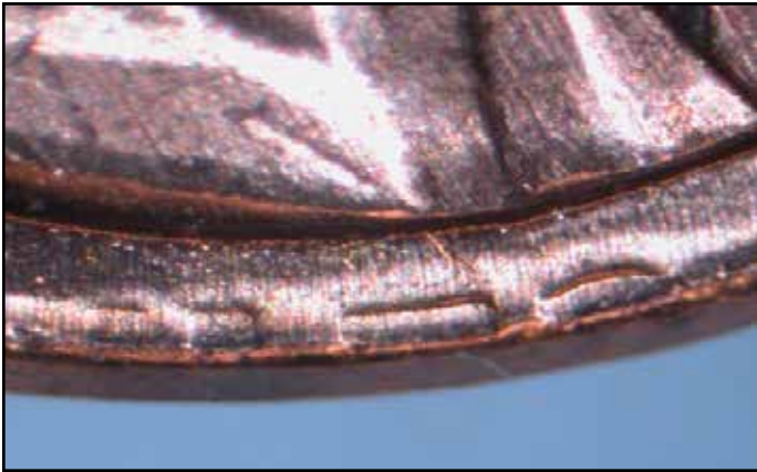
Figure 7. The second of three clashes in this 1997 cent. Letter impressions just inside the design rim indicate die tilt only.
