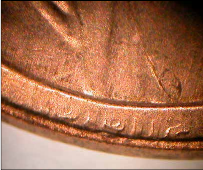
Figure 11. A 2000 cent with a misaligned and tilted die clash located in the gap between Lincoln’s bust and the design rim. This is the only example so far with the misalignment toward the north. Coin courtesy of Bob Mohan.
