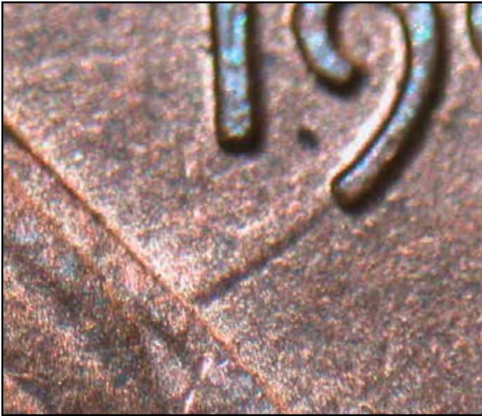
Figure 1. Misaligned and tilted die clash in a 1992 cent. A curved ridge representing the edge of the field portion of the obverse die is located to the left of Lincoln's coat. One or two letter traces are located just inside the curve. Coin courtesy of Richard Imburgia.
