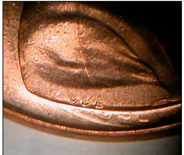
Figure 3. Tilted and pivoted die clash in a 1996 cent.
