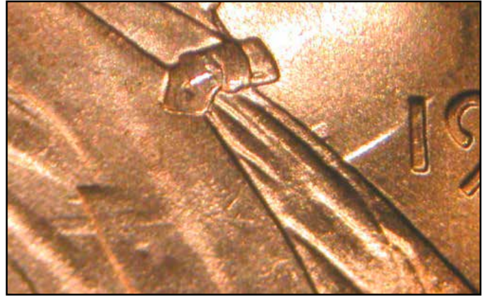
Figure 2. Misaligned and tilted die clash in a 1995 cent. Coin acquired from Mike Ellis.
