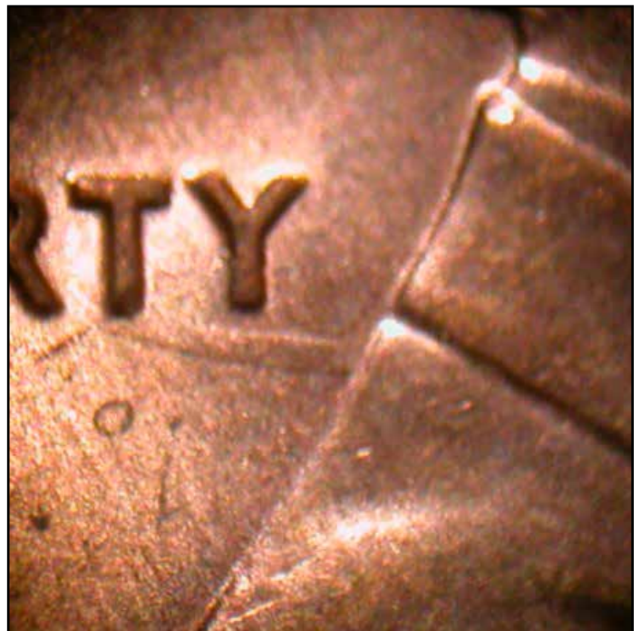
Figure 10. A second 1999 cent with a misaligned and tilted die clash to the left of Lincoln's coat in almost the same position. Coin courtesy of Richard Imburgia.
