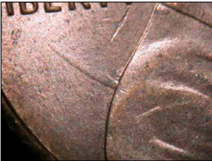
Figure 5. Misaligned and tilted die clash in a third 1996 cent. Coin courtesy of Richard Imburgia.
