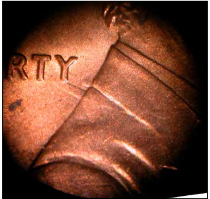
Figure 9. A 1999 cent with a misaligned and tilted die clash to the left of Lincoln's coat. Coin courtesy of G.J. Lawson.
