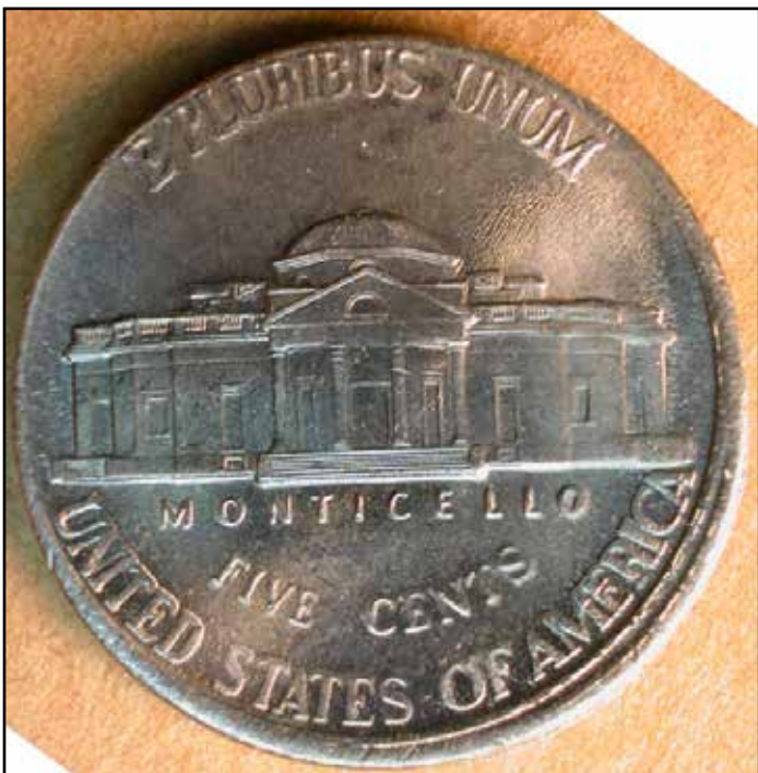
Figure 6a - Reverse face of another 1999-P nickel showing a very clear stutter strike in the southeast quadrant. Coin acquired from Bill Erdakos.
