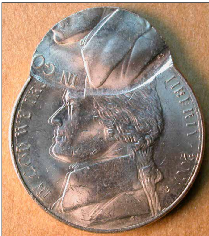
Figure 1a - Obverse face of a triple-struck 2001-D nickel with a horizontal misalignment of the hammer die on the second strike.
