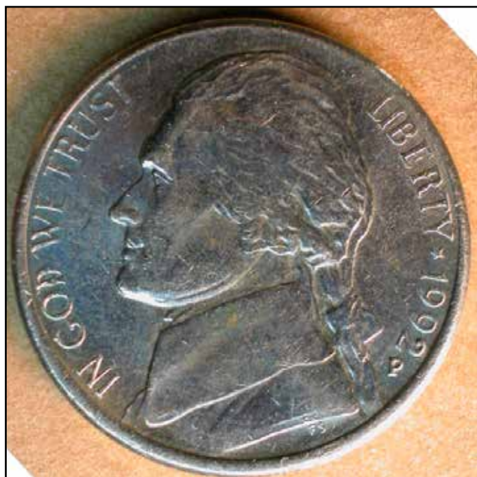
Figure 3a - A 1992-P nickel with severe machine doubling (“push doubling” subtype) on the obverse face. Coin acquired from Mark Westcott.
