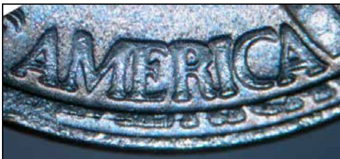
Figure 5c - Close-up of the affected area, showing an extra set of letter tips from AMERICA.
