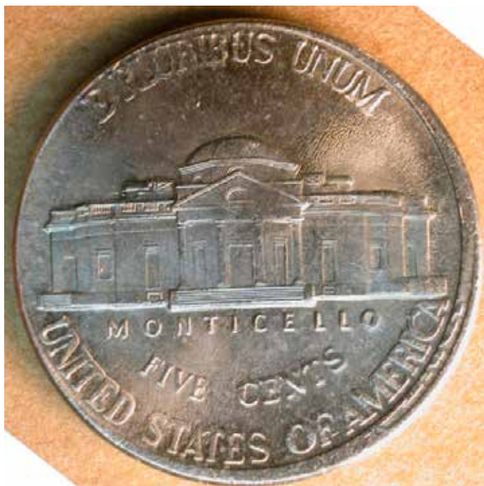
Figure 5a - Reverse face of a 1999-P nickel showing a very clear stutter strike in the southeast quadrant. Coin acquired from Charles Rickard.
