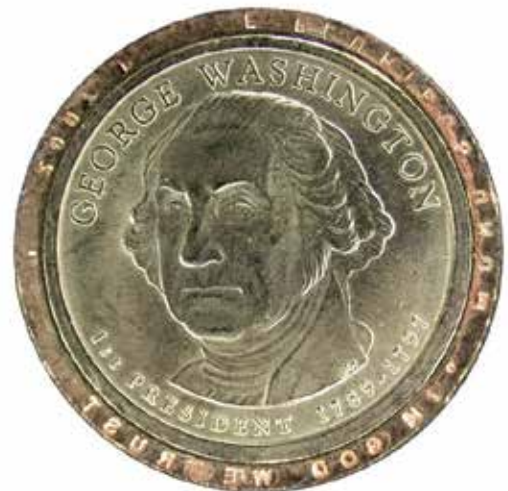
Photo #2b: Improperly spaced edge lettering. Note the irregular gaps between legends.
