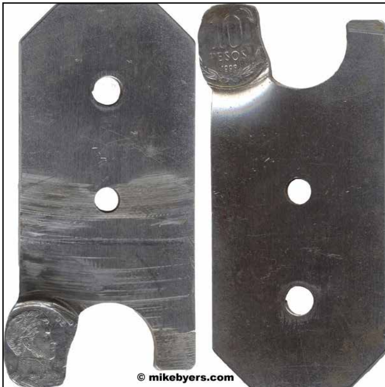
Chile 10 Pesos Double Struck on Feeder Finger
