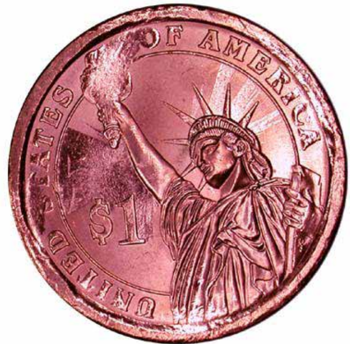
Photo #5b: Reverse missing clad layer.
