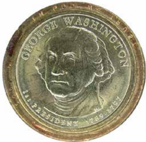
Photo #3b: Partial edge lettering. E PLURIBUS UNUM is missing.
