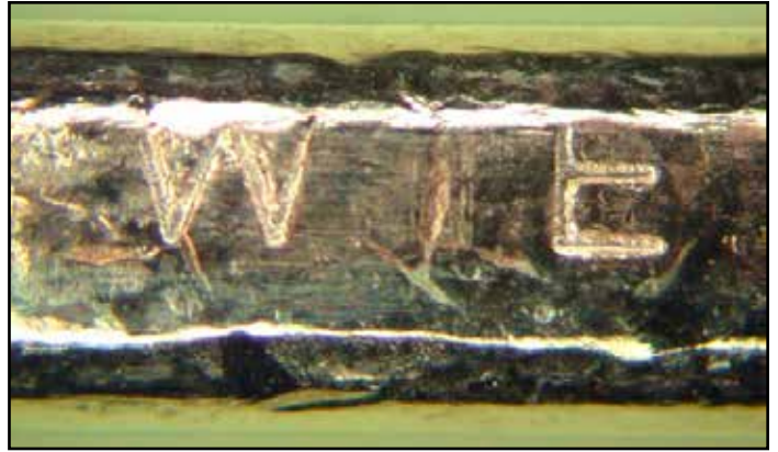
Photo #3b. A portion of edge legend on a Monroe $1 planchet. WE of IN GOD WE TRUST is clearly visible.
