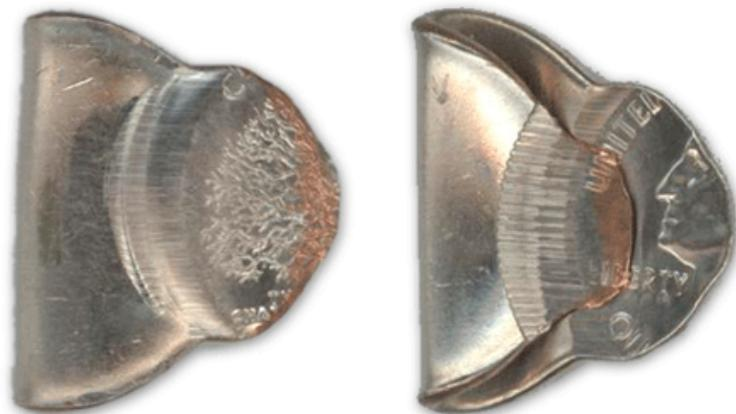
A fold-over coin is one of the most dramatic types of errors. It occurs when the blank is standing vertically between the dies. During the strike, the force is so great that it bends and folds the blank. These fold-overs can be on-center or off-center, and come in many different shapes. There are a few fold-overs with multiple errors, either with an additional strike or fold-over. Denominations above quarters are very scarce.
