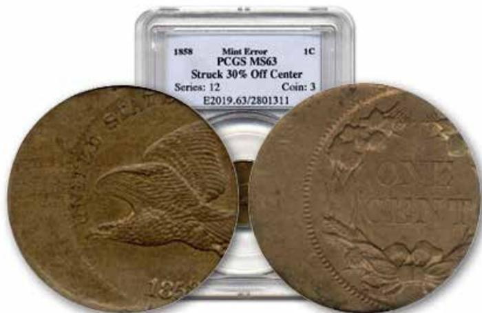
Off-center coins are one of the most common and best known types of errors. This happens when a blank which is supposed to be fed into the press, lands in the collar improperly. When this occurs only part of the blank is between the upper and lower dies. When the dies strike the blank, only that part will be struck with a design.
