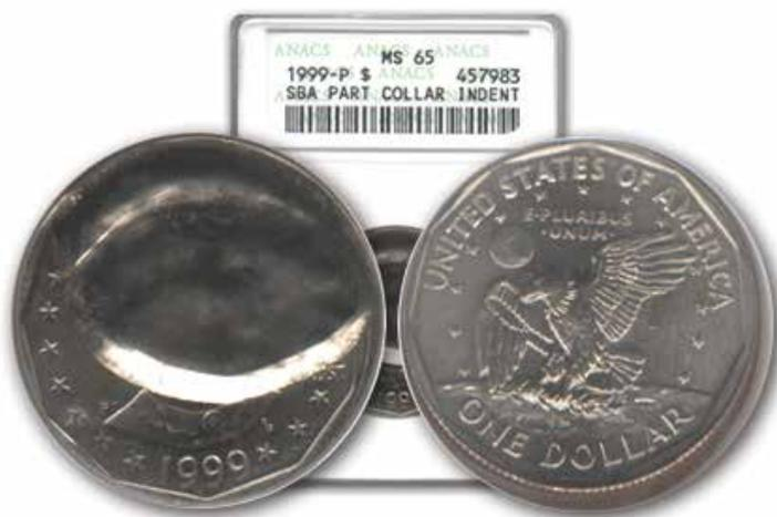
An indent error occurs when two blanks are fed inadvertently into the same collar, with one blank partly overlaying on top of the other. When the hammer die strikes this combination, the upper blank will be forced into the lower blank, creating a depression which is shaped similar to the upper blank. A scarce type of indent occurs when a blank intended for one denomination lands on top of a blank from a different denomination.
