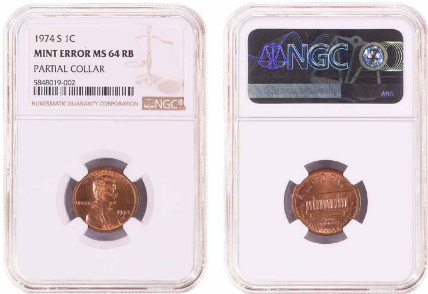
1974-S Lincoln Cent graded NGC MS 64 RB with a Partial Collar Mint Error. Note the uneven thickening of the rims on both sides of the coin.
