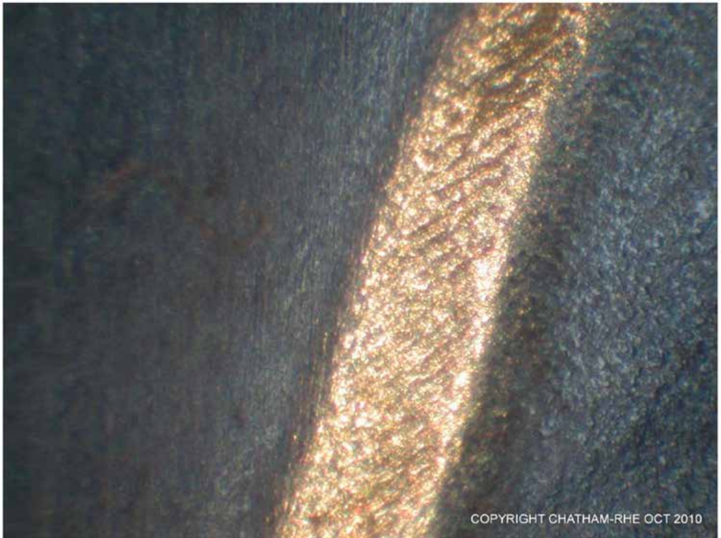
FIGURE 26 This photo is of the edge of Ike’s neck, field to your left. Strong side-lighting was used to bring out the regular pattern left by the burr cutter on the business end of the Janvier lathe. This pattern is present on some of the Obverse edges and more copiously on device edges on the reverse.
